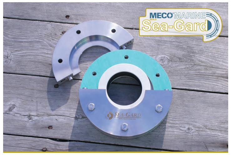
The SEA-GARD provides an effective rudder post seal in abrasive, coastal waters. Wear materials are softer than those used in traditional mechanical seals, and permit the use of wide-radius seal faces. These easily tolerate severe eccentric rotation and permit wear to occur without compromising the seal.
