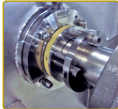
**OFS TYPE-2 SEAL INSTALLED ON A DRY POWDER RIBBON BLENDER**
