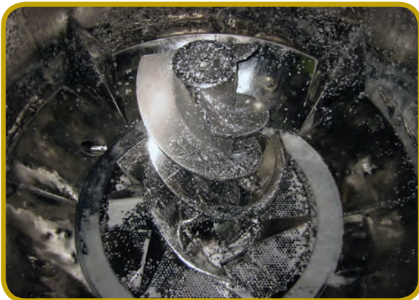
INTERIOR OF 300MM, HI-CON PULPER IN PHOTO ABOVE.
