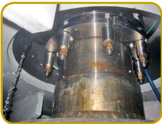
SPLIT EP TYPE-1 ON A PULPER WITH A 280MM SHAFT, PROCESSING OCC.
