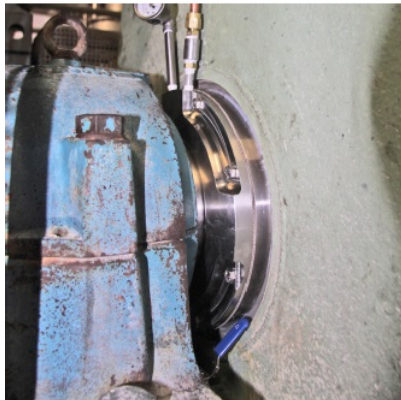
Figure 2. The MECO AH Type-2 model is ideal for fitting a split seal into limited space on small to large shaft diameters containing solids, liquids and vapors. Source: MECO
