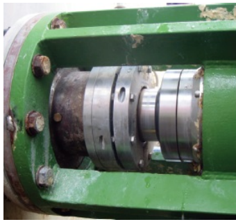
Figure 3. The MECO EA Type-1 fully-split seal model is ideal when sealing wet slurries. Source: MECO
