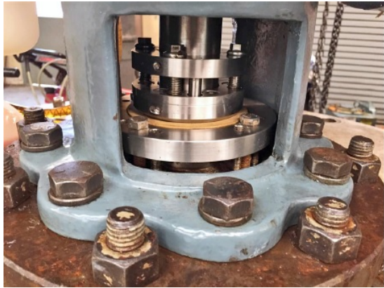
Figure 1. MECO OFS Type-1 split seal permits radial shaft motion on a top entry agitator while providing vapor containment. Source: MECO
