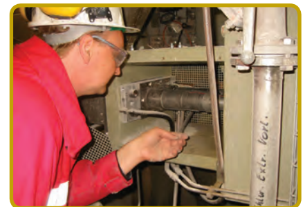
MECO SEAL ON COPERION ZSK-92MC EXTRUDER
