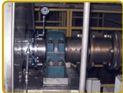
MECO EP T3 INSTALLED ON A VACUUM DRYER.
