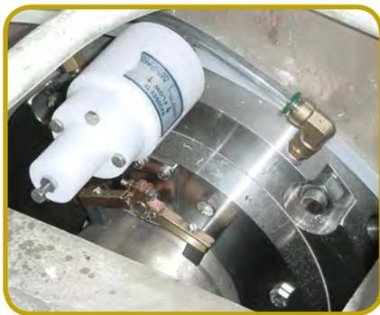
Several MECO seal models are available with ATEX certification. Common to all are a risk assessment, thermal testing and documentation, combined with a variety of protective measures designed to eliminate ignition sources, control surface temperatures and isolate process from atmosphere.
