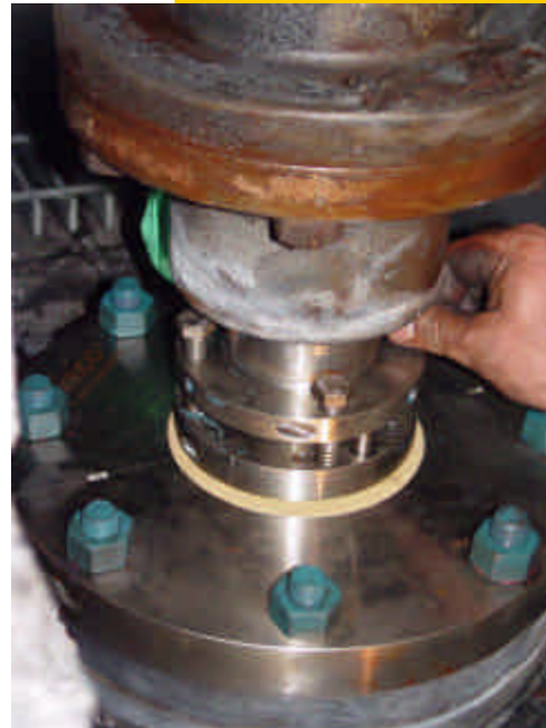
Split OFS seal on 3½" top-entry agitator
