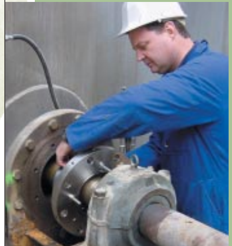
Below: EAS Seals are fully-split for installation without bearing or drive removal.
