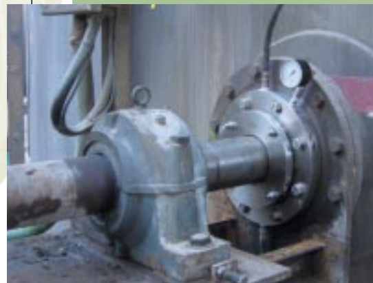
Below: 4 1/2" EAS seal mounted on black liquor agitator
